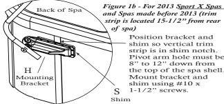
Position bracket and shim so vertical trim strip is in shim notch. Pivot arm hole must be 8" to 12" down from the top of the spa shell. Mount bracket and shim using #10 x 1-1/2" screws.
